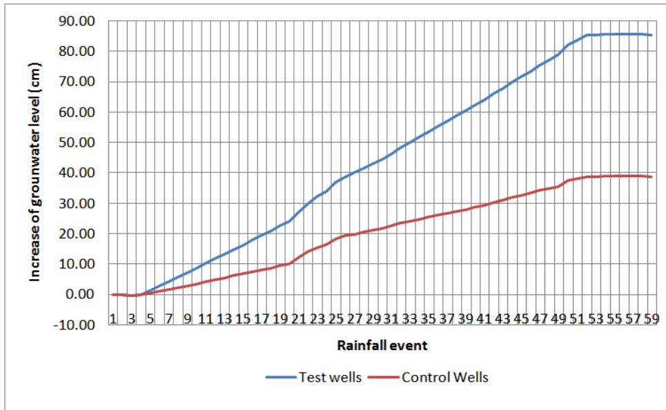
Figure 9: Increase of Groundwater Level in Test Wells & Control Wells (Thickness of Semi-Permeable Layer = 4,00 m)
